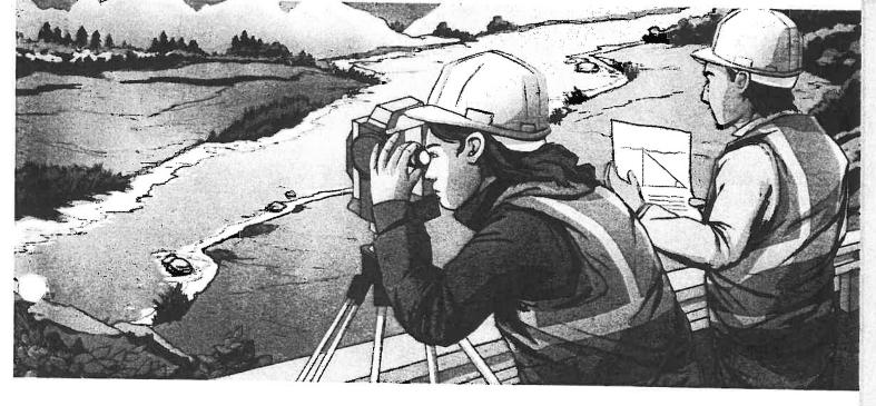
These surveyors are measuring the distance across a river so that a new bridge can be built. Surveyors use **trigonometry** in their work. To measure long distances, they might use a laser measuring device. To measure horizontal and vertical angles, they might use a theodolite—an instrument made by combining a telescope and two circular protractors.
