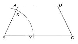
Use the compass to measure XY on the original angle. Then draw an arc with that radius from point Y on the copy. Label X on the copy. Draw a line from *B* through *X*.
